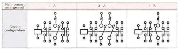
NOTE: The main circuit and coil have no polarity.
